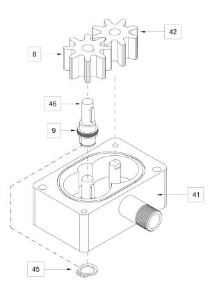
Remove the gear (8 - 42) from the dosing head (41), then using a pliers to remove from its seat the seeger ring (45) located under the dosing head.
